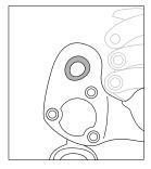
• Check the edges of the attachment hole for wear caused by connectors.
