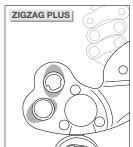
Check the condition of the plastic part, especially in the rope path.
