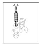
• Check the condition of the positioning ring (deformation, cracks, cuts...). Take care to avoid lubricating this area; it must stay dry to position the carabiner.
