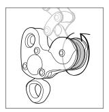
• On pre-2019 ZIGZAG and on the ZIGZAG PLUS, check the condition of the swivel (cracks, deformation...).
