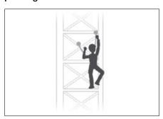
The ABSORBICA-Y lanyards with two arms allow for continuous protection when passing an intermediate anchor, by successively detaching and re-attaching the two arms.
