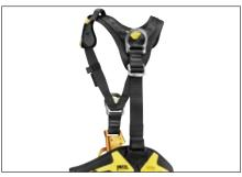
ASTRO BOD FAST full-body harnesses are equipped with a dorsal attachment point for attaching a fall arrest system. In case of a fall on this attachment point, a shortened adjustment of the waistbelt to leg loop length means the load is taken up on the leg loops, allowing the user to remain suspended longer while awaiting rescue.
