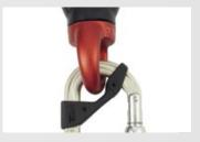
The oval, symmetrical shape allows optimal loading of the carabiner when setting up anchors. Usage with the CAPTIV positioning bar favors loading of the carabiner along the major axis, limits flipping and keeps it attached to the device or lanyard.
