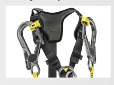
The harnesses have a stowage system for fall arrest lanyard connectors on each shoulder strap. In case of a fall, this system releases the MGO connector and allows the absorber to be deployed.
