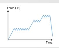
In case of a fall, the tearing of the energy absorber webbing limits the impact force on the user. The lanyards are designed for users who weigh between 50 and 130 kg. The progressive tearing of the webbing reduces the deceleration on lightweight users.
