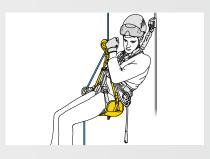
Self-braking descenders are versatile and can be used for both descents and short rope ascents.
