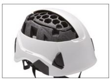
The liner of STRATO helmets is designed in two parts: EPP (expanded polypropylene) and EPS (expanded polystyrene), for reduced weight. Shock absorption is achieved through deformation of the liner.
