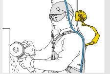
The ASAP'SORBER energy-absorber allows the user to keep the rope at a distance, freeing the work space and protecting the rope (from sharp tools, molten metal splash...).
