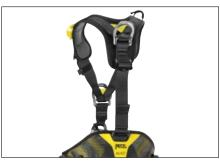
The AVAO BOD and AVAO BOD FAST full-body harnesses are equipped with a dorsal attachment point for attaching a fall arrest system. In case of a fall on this attachment point, a shortened adjustment of the waistbelt to leg loop length means the load is taken up on the leg loops, allowing the user to remain suspended longer while awaiting rescue.
