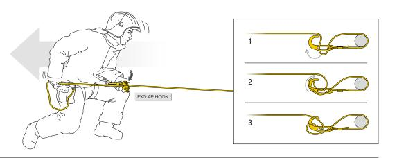
Going through a window while maintaining the anchor hook on the window sill. Locking the left leg against the interior wall to control the movement. Re-establishment below the window while holding the free end of the rope.
