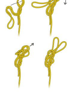
Special case: isolate a section of damaged rope with a butterfly knot.
