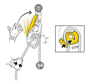
Once locked, the rope can be taken up without having to manipulate the handle.
