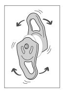
• For pulleys with moving side plates, verify that the side plates rotate properly.
