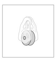
• Check the condition of the sheave (marks, deformation, corrosion, absence of foreign bodies...).
