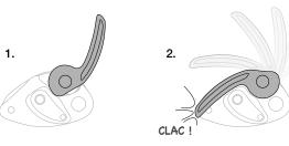
• Check that the handle return spring is working properly.
