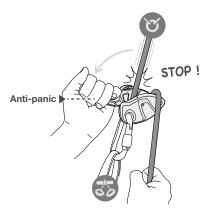
3. Checking the anti-panic on the GRIGRI +. Hang from a low height. Pull the handle QUICKLY while holding the brake-side rope. The rope should be locked.
