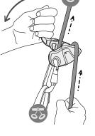
2. Hang from a low height. Pull the handle while holding the brakeside rope. The rope must slide through the device.
