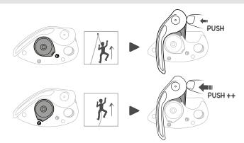
• Check the selector knob for proper function. (When rotated, the cam offers more resistance in the lead climbing position than in the top-rope position).
