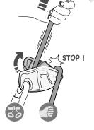
1. Pull on the climber-side rope; the device should lock the rope.
